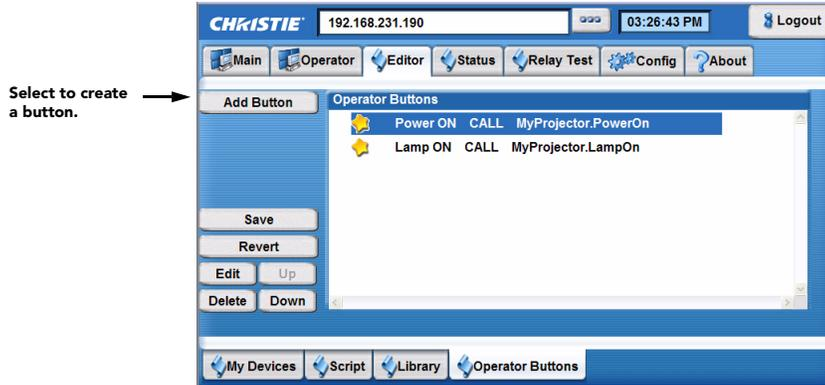
Figure 3-14 Editor: Operator Buttons Virtual Buttons
